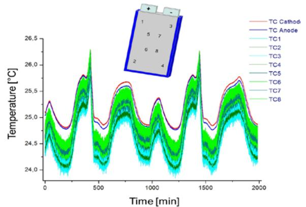
Fig. 4 Surface temperature distribution on a NMC pouch cell during isoperibolic cycling at C/8 rate and 25 °C.
