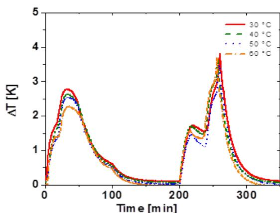
Fig. 1 Temperature difference on a cylindrical 18650 LMO cell during isoperibolic cycling at different temperatures and 1 C rate.
