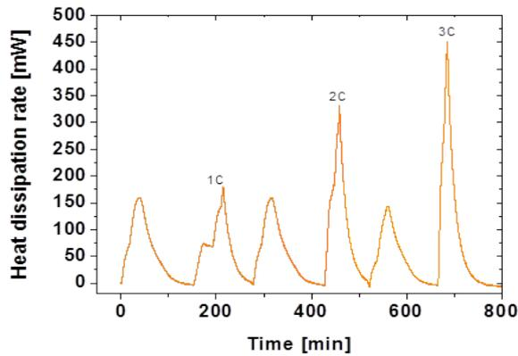
Fig. 3 Comparison of heat dissipation rates at different discharging rates measured on a cylindrical 18650 LMO cell during isoperibolic cycling at 60 °C.
