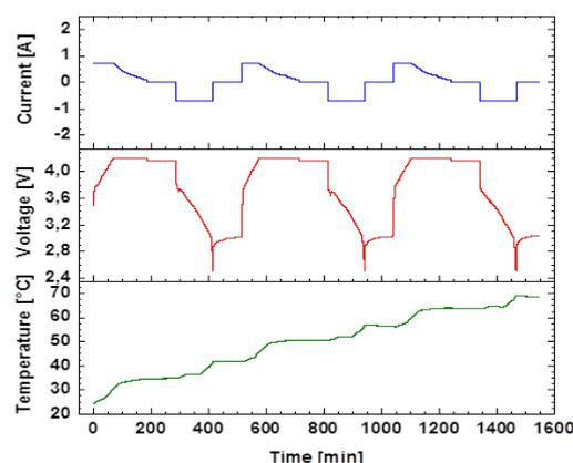
Fig. 2 Current, voltage and temperature curves on a cylindrical 18650 LMO cell during adiabatic cycling at 0.5 C rate starting at 23 °C.
