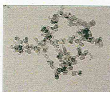
Figure 1) Ship diesel soot (TEM microphotograph) were performed at a wood combustion test facility (KIT) and at a research ship diesel engine which is operable with both, light and heavy fuel oil (L/HFO, U Rostock). The characterization of the aerosols includes a comprehensive chemical and physical profiling (GC-MS, LC-MS, FT-IR, ICP-MS, SMPS, AMS, ELPI, PTR, TEM). The ship diesel exhaust contains soot aggregates (Fig. 1), associated with organic and inorganic compounds. Furthermore two
