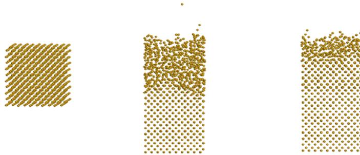
Fig.2 Silicon substrate (left), amorphous silicon coating at high deposition rate (middle), crystalline coating at low deposition rate (10% of the deposition rate in the middle example)
