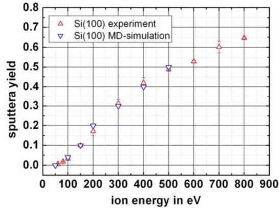
Fig.1 Silicon sputter yield as a function of argon impact energy: comparison between experiment and molecular dynamics simulation
