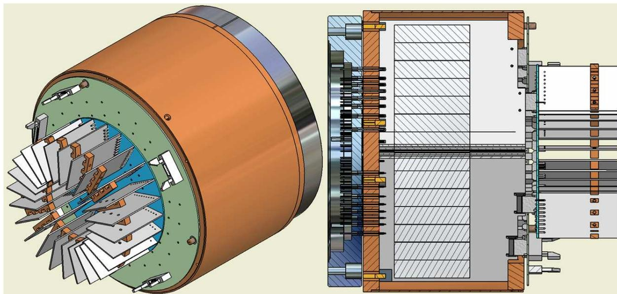
Figure 1: **Focal Plane Detector System** On the left side is an isometric view of the complete assembly as it will be installed. On the right side is a section through this assembly showing the individual components in more detail.
