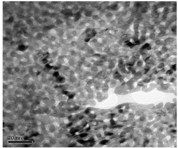
Figure 1: Bright-field transmission electron micrograph of dealloyed gold leaf (Wasner, 6 carat) showing the bicontinuous microstructure consisting of interpenetrating networks of pores and Au ligaments.
