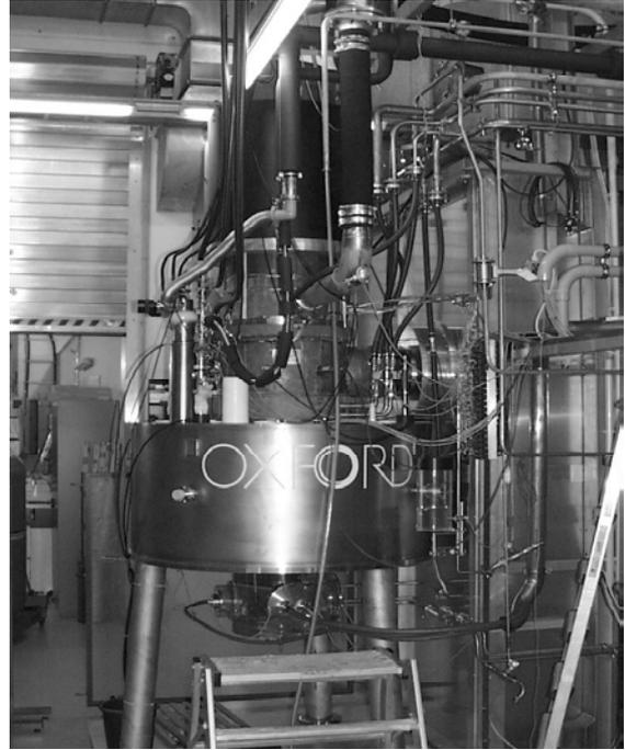
Fig. 1: The gyrotron at the teststand with a view to the microwave chamber
