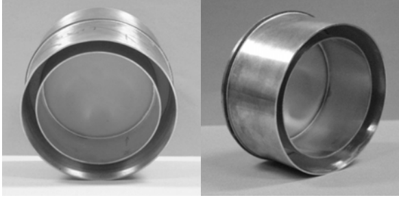
Fig. 4 Basic window disk unit after brazing and removal of the double ring structure at the counter-face.
