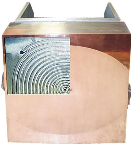
**FIGURE 7:** Single beam mirror with the Cu-SS sandwich structure and cooling channels.
