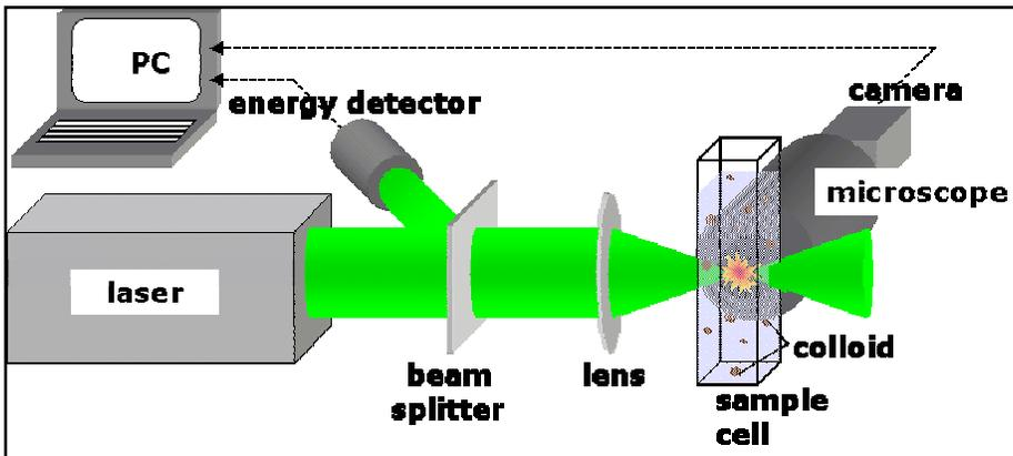
The Laser-induced breakdown detection (LIBD) is a highly sensitive method for the direct detection of nano-particles (colloids). During the detection process plasmas are generated
