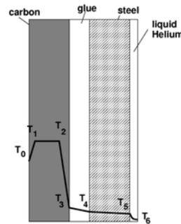
Fig. 1. Cross-section of the panel and corresponding temperature profile.
