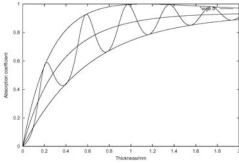
Fig. 2. Absorption coefficient vs. carbon thickness.
